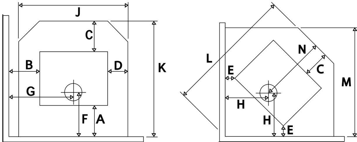
Dimensions 'K' and 'F' are taken from door seal lip (fire box) to the front of the floor protector.
